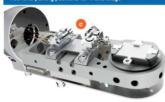
4-axis flag-style heat / cool stage with a 2 level parking stage (c), both electrically floating and coolable which can be loaded from either side:
